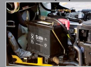
Rotational battery installation
